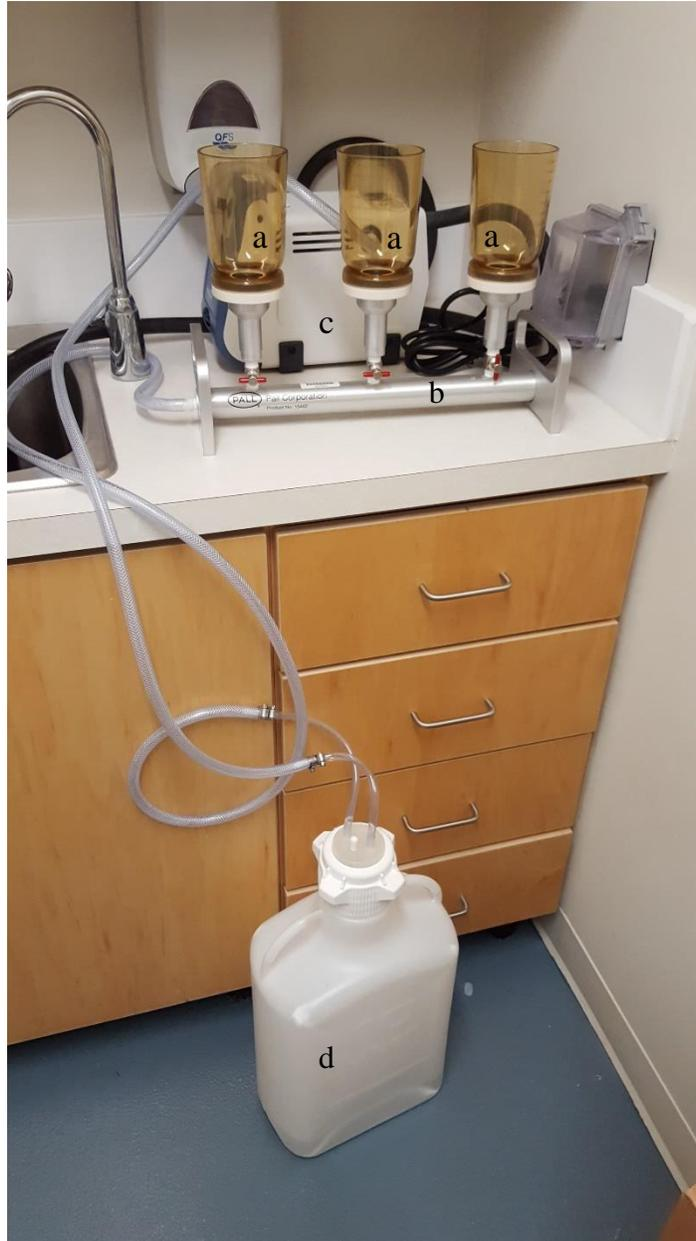
**Figure 1. Filtration set up with 500 mL filter funnels (a) on a 3-place filter funnel manifold (b) which is attached to a dry vacuum pump (behind manifold) (c) and carboy (d) to pump the sample water through filters that are secured at the bottom of the filter funnels and catch DNA and sediment larger than 1.2  $\mu\text{m}$ .**
